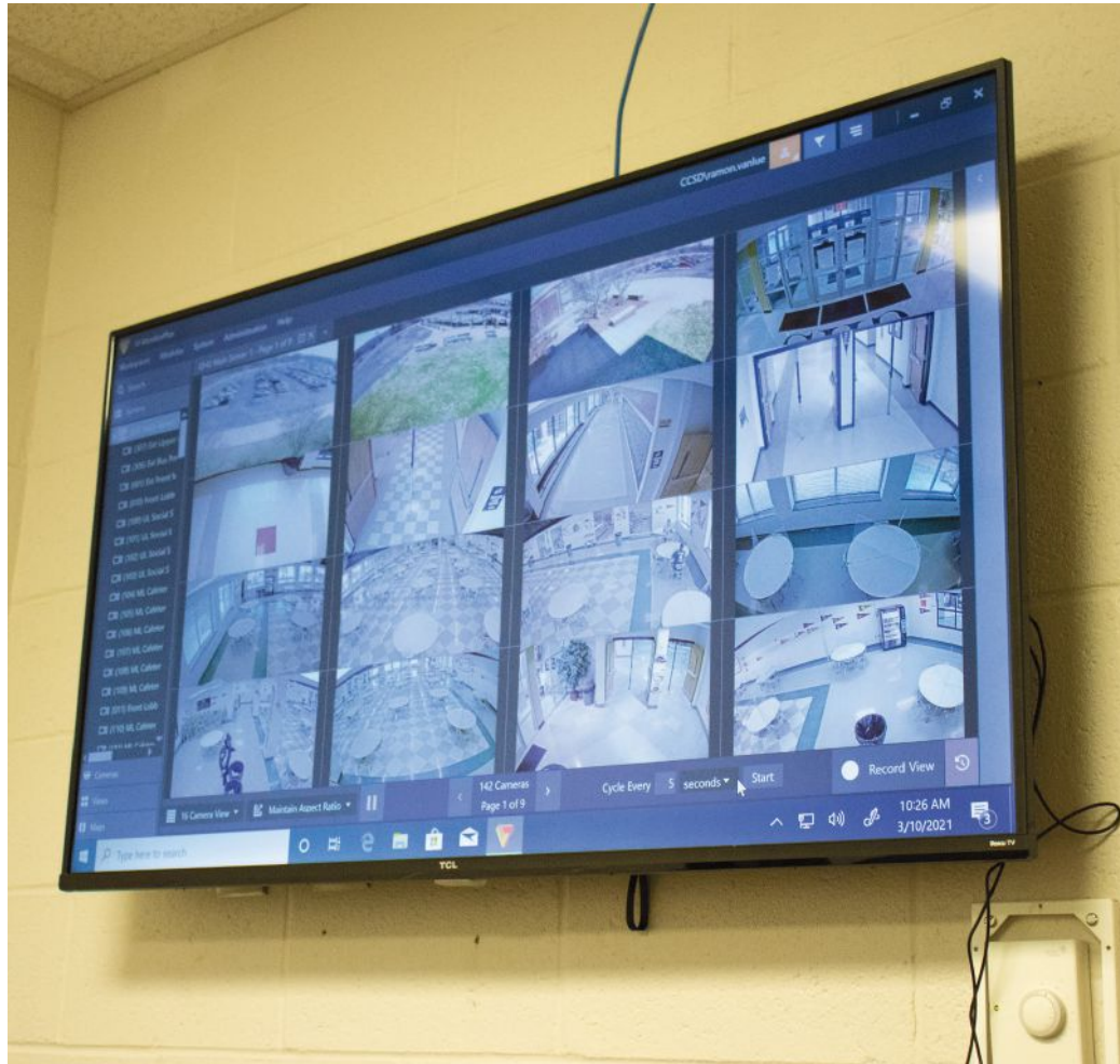
Above: CCSD audio/visual technician Ramon Vanlue monitors the Gaffney High School IP surveillance cameras using Videolnsight's Video Management Software (VMS).
